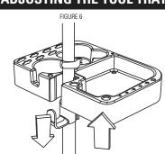
NOTE: To reposition, lift Tool Tray half way off the Tray Mount, slide the tray Mount to new Position and push Tool Tray back down onto Tray Mount
