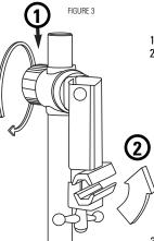
Loosen the Large Hand Knob on the Clamp Arm until it stops.
