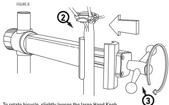
4. To rotate bicycle, slightly loosen the large Hand Knob.5. Rotate bike to desired position and re-tighten.(will not harm the clutch mechanism to rotate under load)
