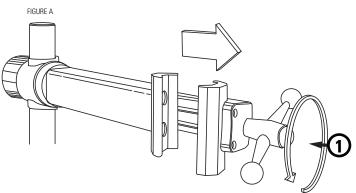
Lift and place seatpost into the clamp against the inner Jaw.
