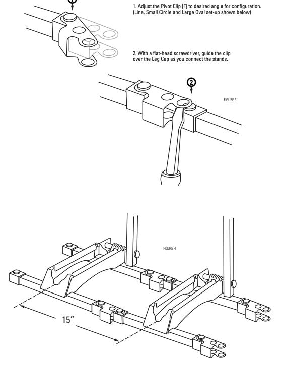
**NOTE:** The different holes on the Pivot Clip allow spacing options of 12", 13.5" and 15".
