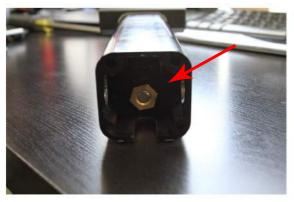
Step 2: Remove 5/8" brass nut from threaded internal rod.
