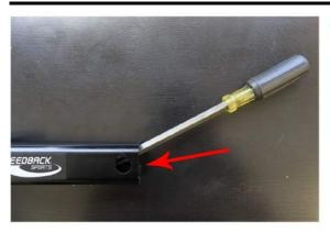
Step 3: Remove cam pocket from clamp head by prying against top of cam pocket from inside.
