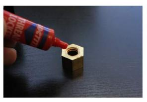
Step 6: Apply red thread locker to inside threads on brass stop nut.
