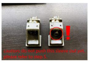
Step 4: Reinstall new cam pocket assembly by inserting into clamp head and pressing upwards until cam pocket snaps into place.
