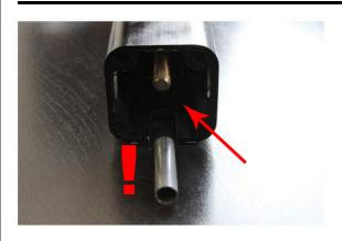
Step 5: Insert threaded rod portion of slide lock jaw through new cam pocket assembly.
